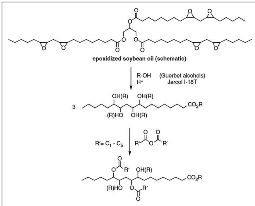
Fig. 3. Base oils from epoxidized soybean oil.
