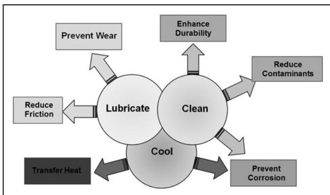
Fig. 4. Lubricants are required to provide three key functions for smooth engine operation and to improve longevity: to clean, cool and lubricate.
