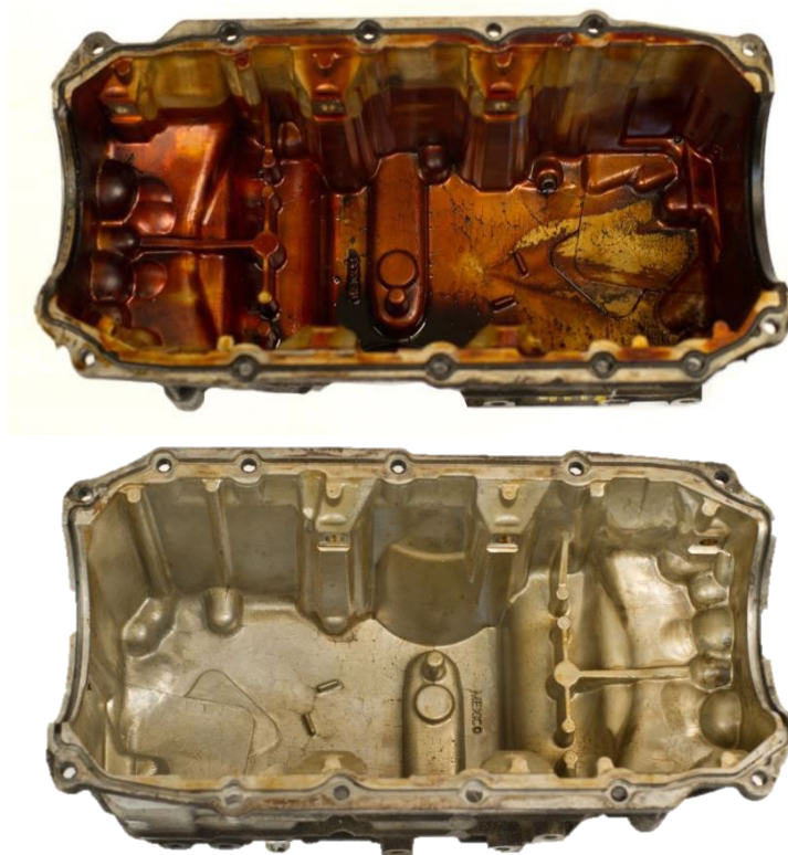
Figure 10 – Oil pans from two Chevy Impala 3.5 liter V6 engines used in an 18 month 150,000 mile field trial in Las Vegas, NV. The conventional motor oil formulation (top) had a typical level of varnish at the end of the test, while the estolide formulation (bottom) showed a high degree of overall cleanliness and minimal varnish.
