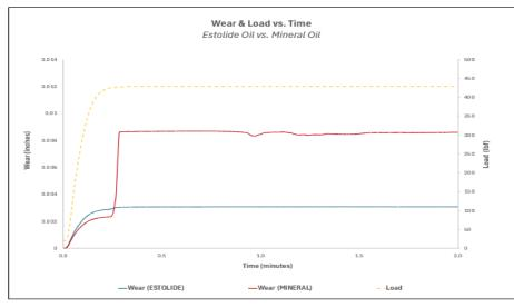
The lower the wear value, the better performance of the drawing and stamping process that consistently leads to higher quality finished metal work pieces, longer tool performance, and tool longevity.
