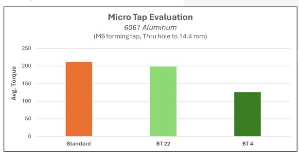
The standard used for comparison was a heavy duty semi-synthetic metalworking fluid containing a Phosphate EP additive. The phosphate additive was replaced by BT 4 and BT 22 at 15%. As you can see, the BT 22 sample reduced torque by 10% leading to better performance on aluminum.
