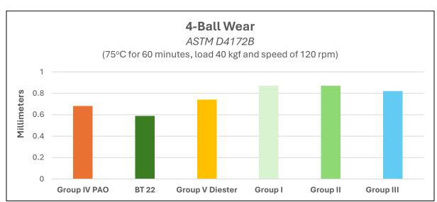
The test above was run to compare various base oils in a 4-ball wear test. As you can see, BT 22 performed better than a low viscosity PAO and much better than Group I, II, III and V base oils.
