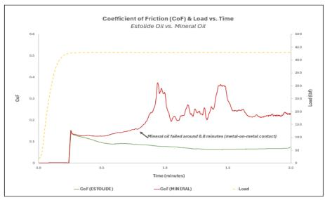
Lower CoF values promote enhanced tool life and higher quality machining of work pieces. The BT 22 formulation significantly outperformed the mineral oil formulation, which failed the test around 0.8 minutes.
